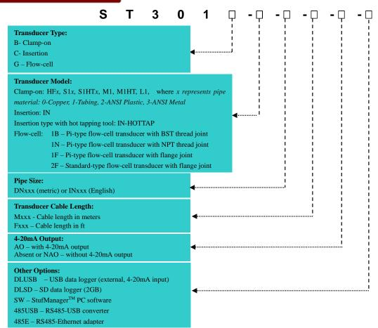
Example: Model# ST301B-M1-DN100-M5-AO stands for economical flowmeter with M1 clamp-on transducer for pipe size DN100mm. 5 meter transducer cable. 4-20mA output.
