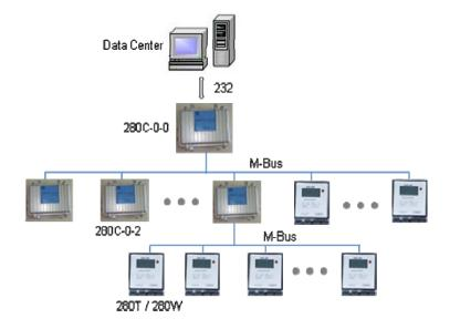
Hierarchical topology of an AMR system using a BACnet concentrator.
