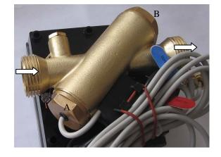
competitors put a sound reflector in the pipe to get a V-shape path or even put two sound reflectors to get a U-shape path. The problem with the reflector is when the liquid in pipe gets dirty, which is quite common in real heating/cooling loop after many years operation, the reflector surface is not smooth anymore and its reflecting efficiency becomes very poor. This could cause the heat meter accuracy largely degraded, or even cause the meter fail to register.
