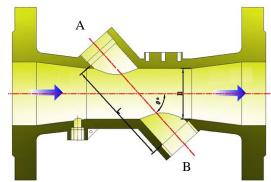
Depending on the pipe size, there are two kinds of transducer arrangement. For large pipes, a straight-through design, as shown in the figure above, is recommended. However, for small pipes, the straight-through does not provide enough sound path to obtain good accuracy. To increase the sound path, our
